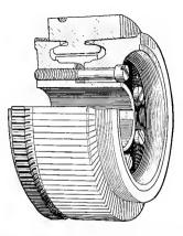
F1G. 83. View and section of a commutator (G. E. Co.), showing segments, collars, insulation, etc.
